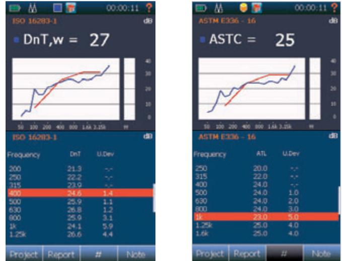
The rating picture for impact insulation. Split screen with graphical and numerical values. If more than one loudspeaker or tapping machine position have been measured, you may use the softkey '#' to scroll through the individual calculated results for each position named A, B, C, ..... The total result is called 'Total'.
