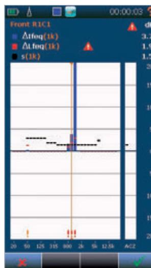
The  $\Delta$ -view shows the difference between two orthogonal scans, in terms of both leq and Leq. Additionally the ISO requirement is plotted in black color.
