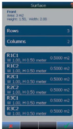
The surface edit menu provides access to all segments inside the surface. The summed area of all segments is displayed. The number of segments may be controlled by editing the Row/Column setup.
