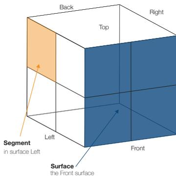
The total measurement surface is divided into several surfaces and segments. Define the overall dimensions, and let the Nor150 auto-generate the complete surface.
