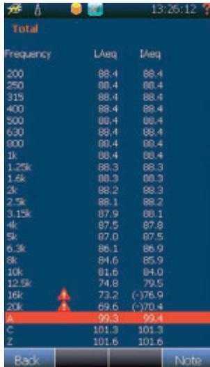
All functions are available in tabular format, including warning indicators. It is also possible to display surface/segments overviews in tabular format, including navigation using double-taps.
