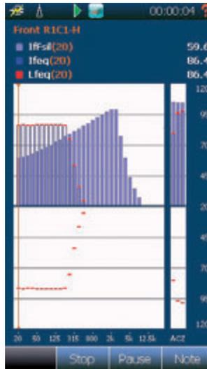
The instantaneous view during measurement. Instantaneous intensity with time constant Fast is displayed along with leq and Leq. Instantaneous intensity is a great tool for localising noise sources.
