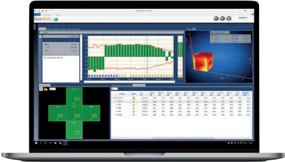
In the Nor850 software you can change all settings the same way as in the Nor150. However, copying and analysing the measurements is easier on a larger screen. The Nor850 software provides intuitive visual tools for editing.
