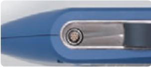
On the right hand side is the power socket, Trigger input and output for synchronized sampling of several Nor150. Also the Norsonic standard 15 pin digital I/O hosting a high speed RS232 interface, 3 digital input, 4 digital outputs, Signal generator, AC output, SPDIF and 3,3Vdc - 50 mA power for auxiliary equipment
