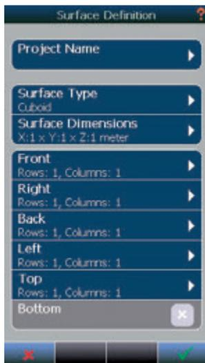
The surface definition menu provides access to the measurement surface setup. Submenus for each surface allows further configuration.
