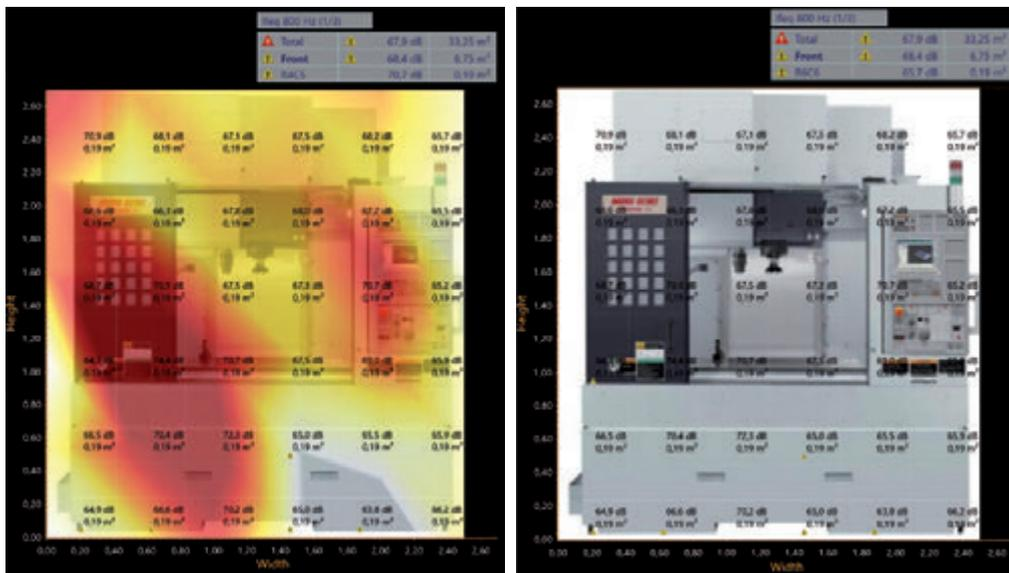
The 2D surface may also display a background picture. To the left: surface information, background picture and color range adjusted for high visibility of small variances. To the right: Color range set to disable color overlay; only segment information is visible on top of the background picture.
