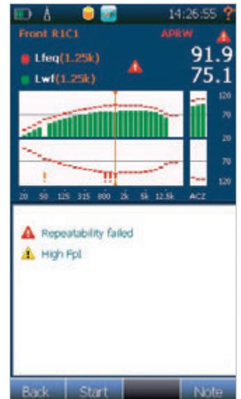
The INFO key will bring up detailed information about the cursor position. Here, A-network preweighting is also applied to the measurement spectra, giving the user a good indication of which band that contributes to the total A-weighted value.
