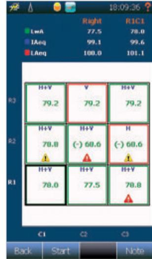
Double-tapping into a surface will show all segments inside the surface. Warning indicators are shown along with scan progress color frame. Key levels are available at the top.
