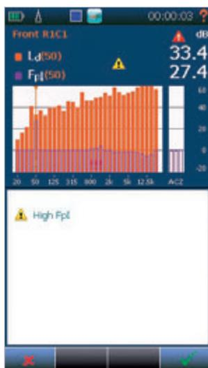
Dynamic capability analysis shows the dynamic capability of the probe and instrument, along with the field indicator Fpl from the current measurement
