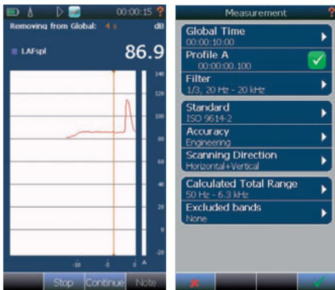
Pressing the PAUSE button will bring up the level-time graph. Move the cursor to remove a desired number of seconds from the measurement, and press continue. The functionality is also available on the remote control.
