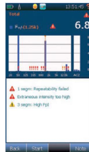
The Extranous Intensity view shows the F+/- indicator for the total surface, displaying the effect of extraneous noise on the measurement.
