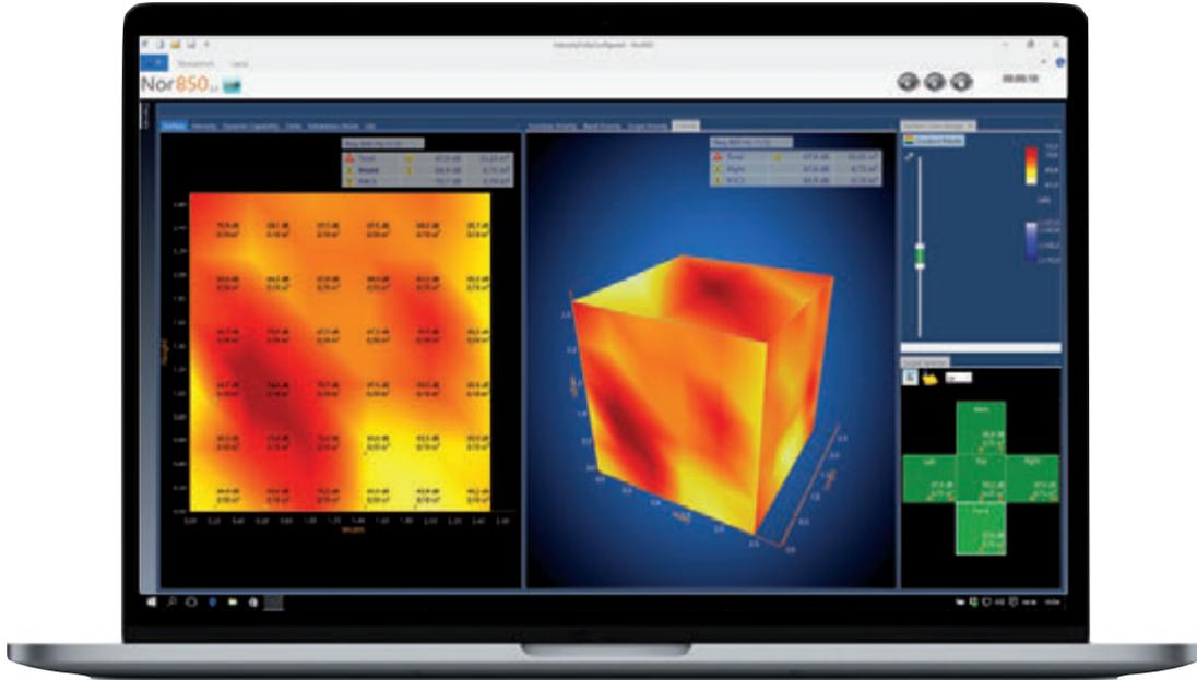
Rearrange the Nor850 to suite your needs. In this case, we have chosen to look at the 2D surface and 3D surface together, along with the Scope Selector and color range adjustment pane. We have also activated the segment information on the 2D surface.
