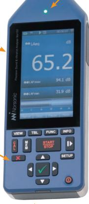
Built in LAN, USB A and mini B connectors, Micro SD card and Headset connector for voice comments and audio recording playback. WLAN and GPRS/3G-4G modems through USB.
