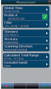
All settings may be changed during or after a measurement, except the baseline Filter settings. Using the calculated total range setting to decide frequency range, all data is kept for optional use later.
