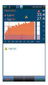
Dynamic capability analysis shows the dynamic capability of the probe and instrument, along with the field indicator FpI from the current measurement
