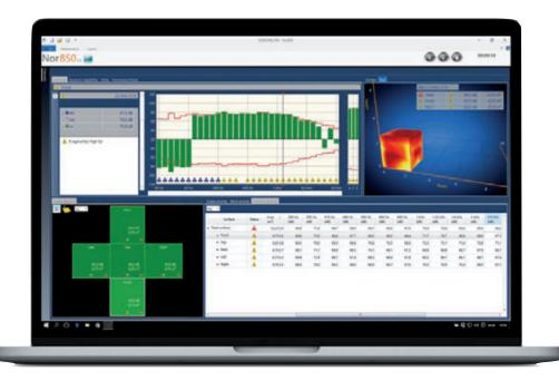
In the Nor850 software you can change all settings the same way as in the Nor150. However, copying and analysing the measurements is easier on a larger screen. The Nor850 software provides intuitive visual tools for editing.
