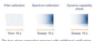
The two-stage correction process with additional verification saves considerable time compared to traditional methods
