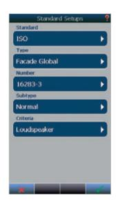
Setup menu for selecting standards. You may recalculate for additional standards based on already measured data.
