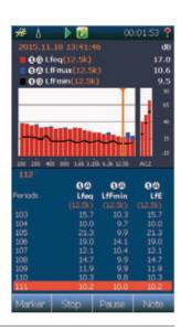
A numerical table is associated with all the graphical views. Just press the TAB button to toggle between graphical and numerical view. Works both with single and split screen.
