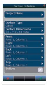
The surface definition menu provides access to the measurement surface setup. Submenues for each surface allows further configuration.
