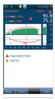
The INFO key will bring up detailed information about the cursor position. Here, A-network preweighting is also applied to the measurement spectra, giving the user a good indication of which band that contibutes to the total A-weighted value.
