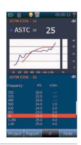
The rating picture for impact insulation. Split screen with graphical and numerical values. If more than one loudspeaker or tapping machine position have been measured, you may use the softkey '# to scroll through the individual calculated results for each position named A, B, C, ..... The total result is called 'Total'.
